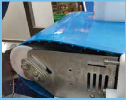
UHMW roundel mounted on pulley
