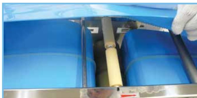
Centre drive narrow transfer with welded bottom guide
