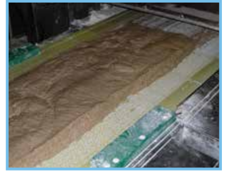
UHMW pieces holding 3mm Volta belt
